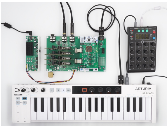
Figure 1: Overview of the synthesizer setup. Top left: custom power supply; top middle: \pm synth hardware prototype; top right: MIDI controller; bottom: MIDI keyboard.
