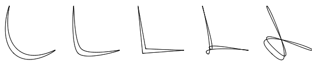
Figure 4: Closed loop tensioned Catmull-Rom splines with four points in an irregular non-convex L-shaped arrangement. \tau = -1, 0, 1, 2, 5 from left to right. The center configuration corresponds to a linear connection between control point positions.
