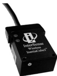
Figure 8: IMU for head-tracking
