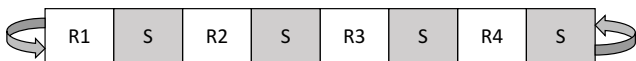
Figure 3: Round robin sampling for training. S is the synthetic dataset and RN are the real datasets: 1:RBM-13, 2:IMDT-SMT, 3:ENST, 4:MDB
