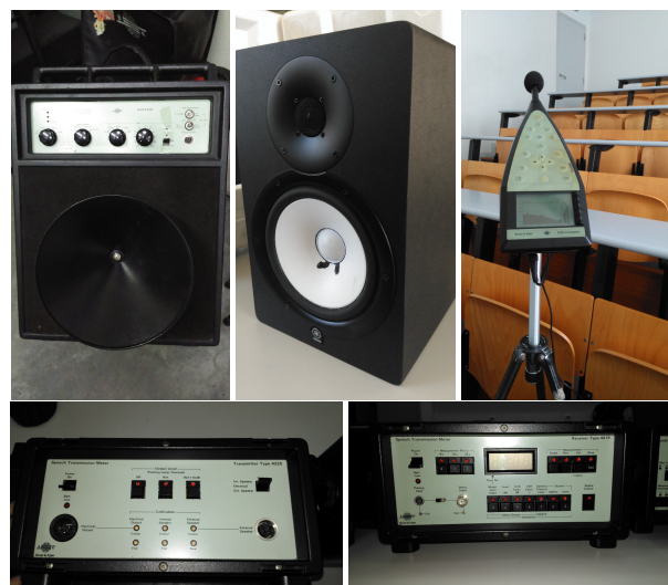
Figure 4: Material used for the measurements. From left to right in the top row are two sound sources and a sound-level meter. In the bottom row are a RASTI emitter and a RASTI receiver.
