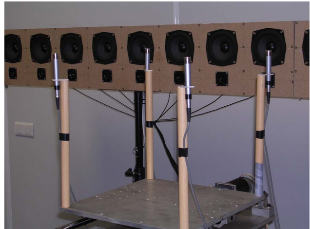
Figure 3: Setup of WFS array and the measuring microphones mounted on the positioning system.
