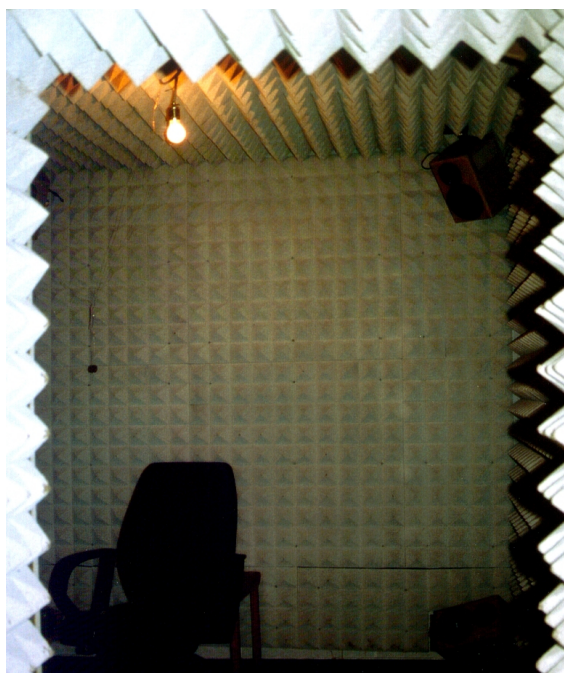
Figure 1: Room with non-reflecting walls as it is used for the realization of a diffuse sound field.
