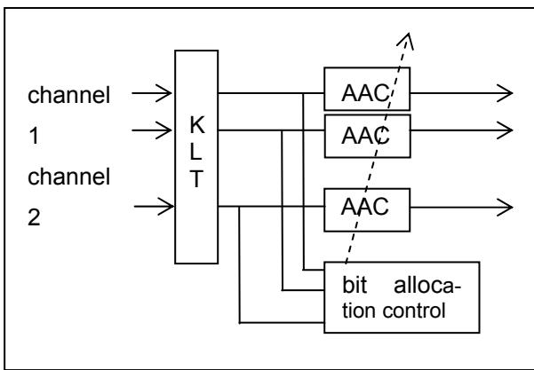
Figure 3: KLT+AAC multichannel coding
