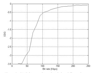
Figure 8: ODG for one channel coded at different bit rates
