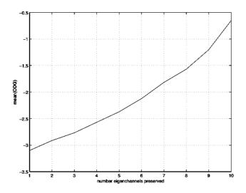
Fig 6: *Mean ODG versus n° of preserved eigenchannels* As we can see, the relationship between quality and number of preserved eigenchannels follows a monotonic increasing law. This property assures that the quality will not suffer a quick fall as we discard eigenchannels. However, it is clear that, with this approach, the quality suffers from a noticeable degradation even if only one eigenchannel is discarded.
