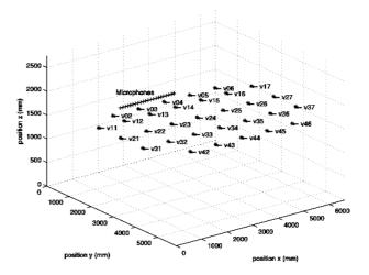
Figure 1: Position of the microphones and the speakers at the varecoic chamber
