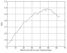
Figure 9: Mean quality after distributing bits after eigenchannel energy
